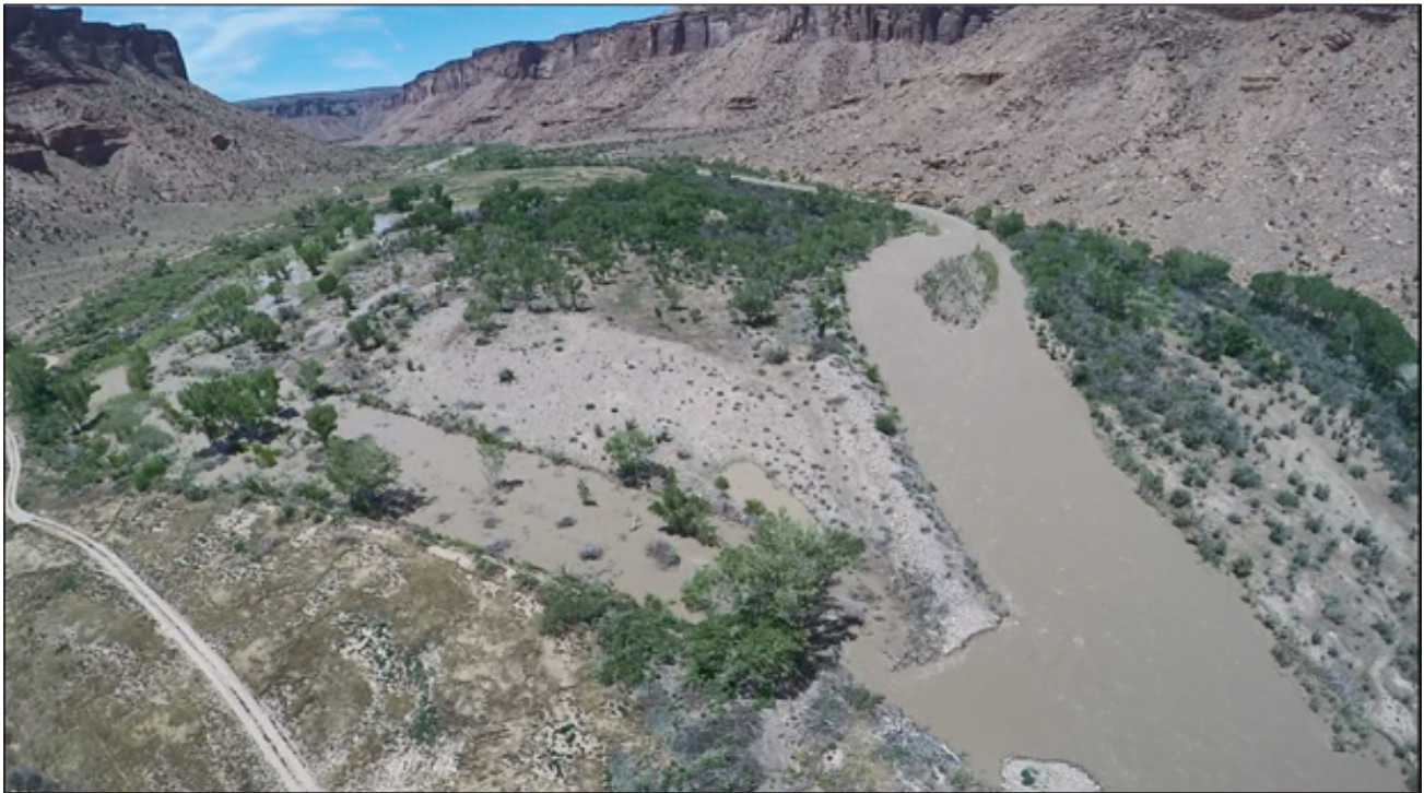
Figure 4. Inundation on June 17, 2019 at ~5400 cfs at upstream berm removal area.
