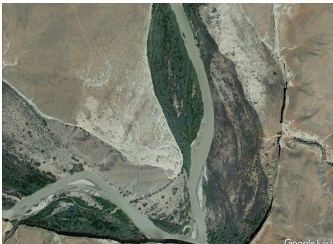
Figure 18. May 3, 2017 photo of project area showing channel narrowing and vegetation encroachment on the river channel.
